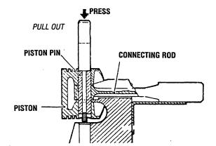
Heat the piston to  $122^{\circ} - 158^{\circ} F (50^{\circ} - 70^{\circ} C)$ .
