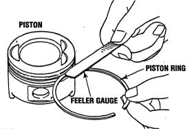
**NOTE:** If replacing piston rings check the piston ring gaps. New rings are packaged with detailed instructions that often supersede the service manual.
