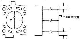
CYLINDERS INSPECT FOR CRACKS, SCORES, OR RIDGES AT TOP OF RING TRAVEL
