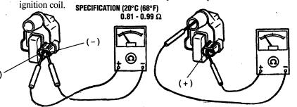
**Secondary Coil Winding:** Measure the resistance at the secondary coil using an ohmmeter. If not specified, replace the ignition coil.
