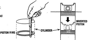
Measure the piston ring to ring clearance around the entire circumference using a new piston ring. CLEARANCE TOP: 0.03-0.07mm (0.001-0.003in) SECOND: 0.03-0.07mm (0.001-0.003in) MAXIMUM: 0.15mm (0.006in)
