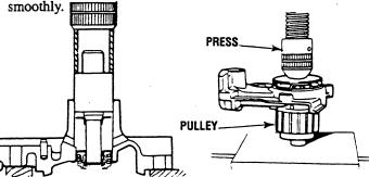
4. Push the pump pulley into place using a press.
