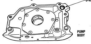
3. Coat the lip of the oil seal with fresh engine oil. When installing the oil seal, be careful not to damage the lip. Tighten the bolts to the specified torque.
