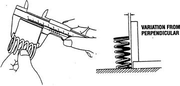
FREE LENGTH EX: 52.2mm (2.0 in) IN: 47.7mm (1.88in) ANGLE EX & IN: 1.8mm (0.07in) MAX
