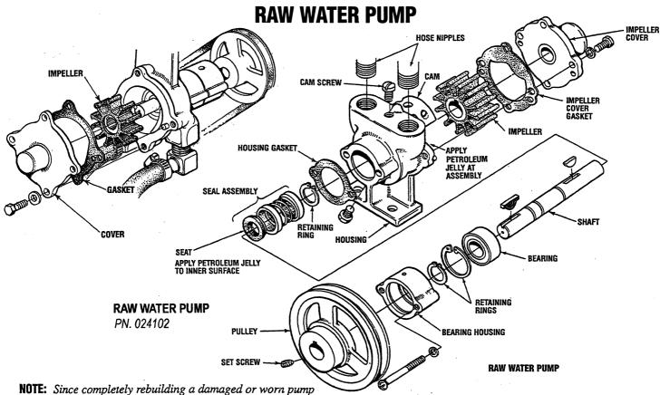
**NOTE:** Since completely rebuilding a damaged or worn pump from individually purchased parts would almost match the price of a new pump, Westerbeke recommends that a new pump be purchased.
