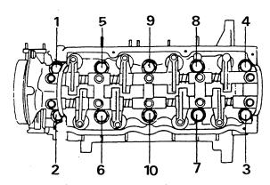
1. Loosen the cylinder head bolts in several increments to remove, following the numerical sequence indicated above.
