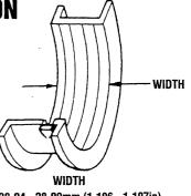
UNDERSIZE PARTS 0.25mm (0.009in) 0.50mm (0.019in) 0.75mm (0.029in) STANDARD
