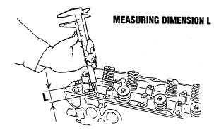
7. Measure the valve stem to guide clearance. (1) Method
