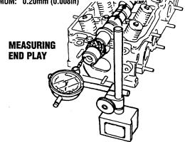
**NOTE:** If the end play exceeds specifications, replace the camshaft and/or cylinder head.
