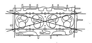
If the cylinder head distortion exceeds specification, grind the cylinder head surface.
