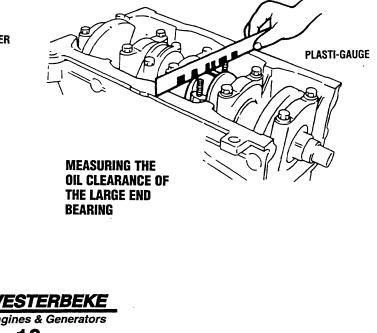
g. If the oil clearance exceeds the limit, replace the bearing set with a new one and measure again.
