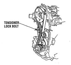
**CAUTION:** Water or oil on the timing belt severely reduces the service life of the belt. keep the timing belt sproket and tensioner free of oil and grease. These parts should never be cleaned. Replace if seriously contaminated with dirt or oil. If oil is evident on these parts, check the front case, oil pump seals, and camshaft oil seals for a possible leak.
