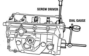
1. Check the end play by moving the crankshaft forward and backward as shown using a magnetic base and dial gauge to measure the amount.
