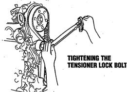
If re-using the same belt, measure the belt tension between the crankshaft pulley and the camshaft pulley. repeat steps if the belt tension is not within specified range.
