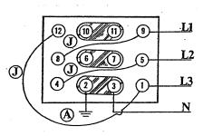
L-L – 450 VAC 3Ø 60 Hz L-N – 265 VAC 1Ø 60 Hz
