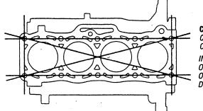
CYLINDER BLOCK CHECK FOR WARPAGE ON TOP FACE INSPECT FOR CRACKS, OIL OR COOLANT LEAKS. CLEAN OFF SCALE AND CARBON DEPOSITS
