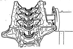
5. Install the main bearing caps in accordance with the numbers and arrows and tighten the bolts to the specified torque.
