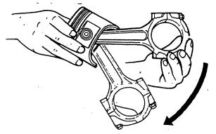
5. After pressing the piston pin in, swing the large end of the connecting rod upward and release it. The connecting rod must swing downward freely.
