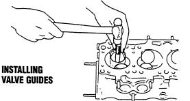
3. Fit the clip onto the valve guide. Use the valve guide remover and installer to tap the valve guide in from the side opposite the combustion chamber until the clip just contacts the cylinder head. The height of the valve guide must be 19.1—19.6mm (0.752—0.772in) from the valve spring seat to the end of the valve guide (dimension A).
