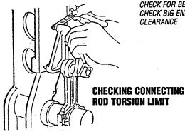
CHECK FOR BEND OR TWIST. CHECK BIG END THRUST CLEARANCE
